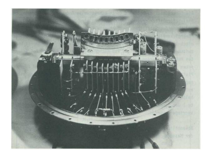
Figure 8: Here also the cylinder part of the housing, as well as the spherical shells by I1a are removed. The channeltrons are carried by a common shaft, on which side the boards with the high voltage cascade are attached.
