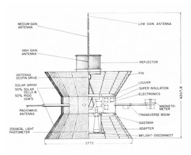
Figure 3: A diagram showing the construction of HELIOS
