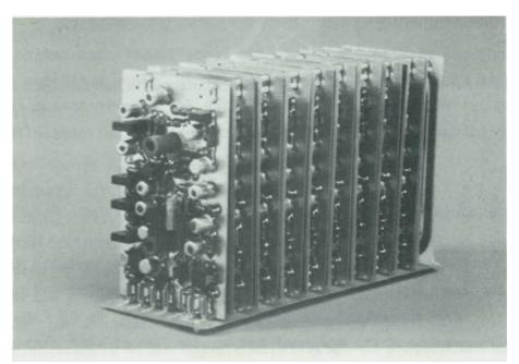
Figure 36: Channeltron amplifier block
