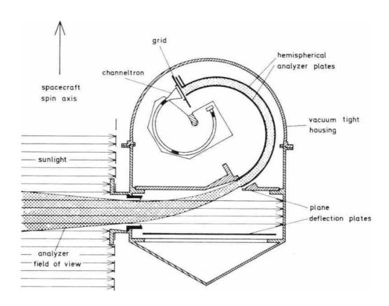
Image 11: Function image of the electron instrument I2
