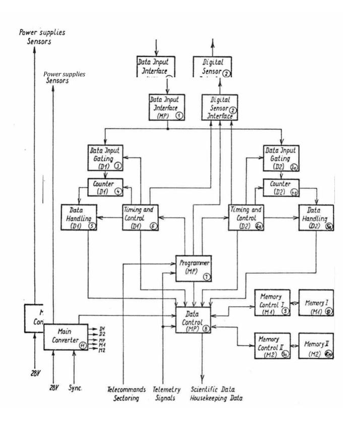
Figure 19: electronic box, block diagram
