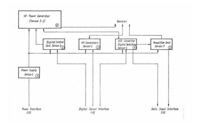
Figure 16: Instrument I3, electronics block diagram
