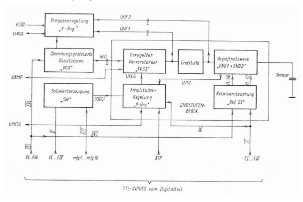
Figure 31: high frequency generator for I3, block diagram
