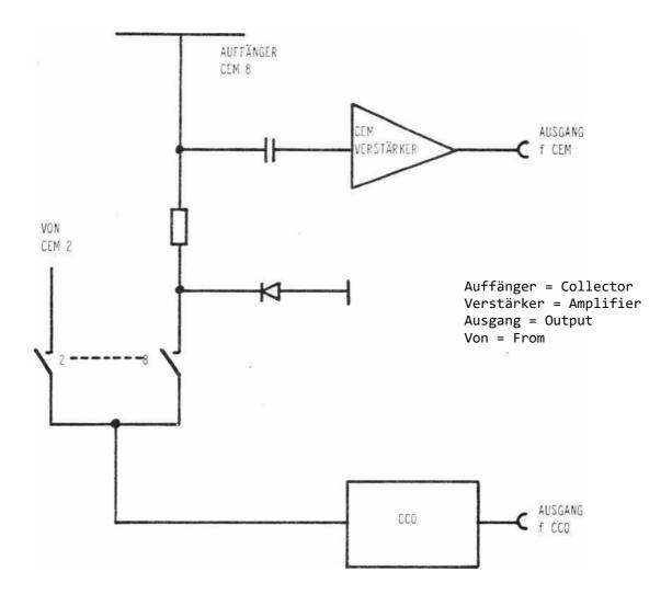
Fig. 30: Amplification measurement of channeltrons
