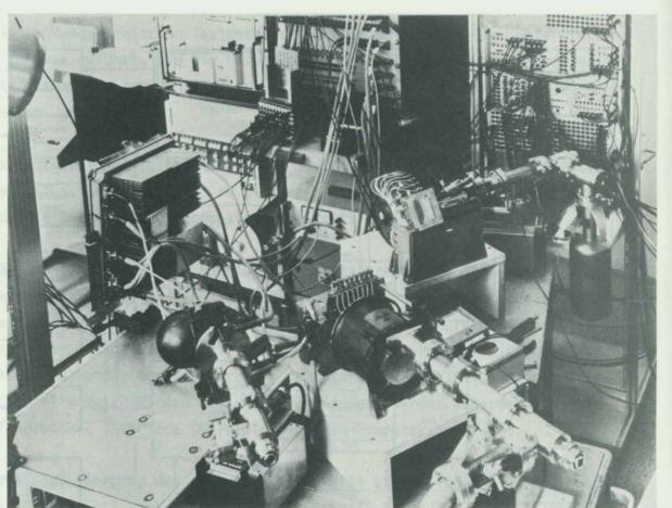
Figure 52: The test device at one of the first total tests of the engineering model of E1.Far left above the teletype for control and data output, in addition the process computer (HP 2100).Top center the "breakout box" for all instrument cables.Right the unit for "hand-controlled" special tests.
