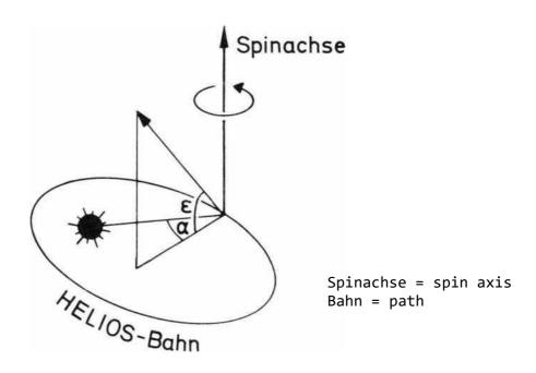
Figure 5: Definition of the angle  $(\alpha)$  azimuth and elevation  $(\epsilon)$  of the particle incident direction.
