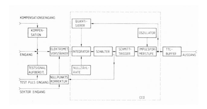
Fig. 27: Electrometer for I1b, block diagram
