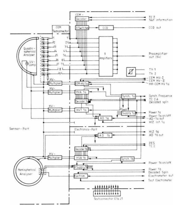
Figure 9: Instrument I1a/I1b, block diagram. The sensor part in the vacuum sealed package contains all parts carrying high voltage, the electronics part analog and digital electronics.
