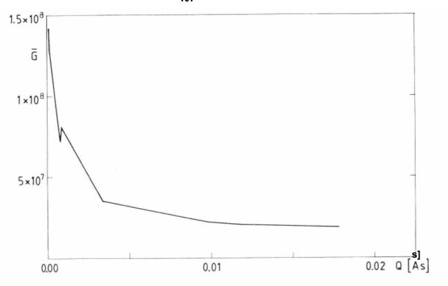
Figure 43: The dependence of the average gain  $\bar{\mathcal{G}}$  of the total charge Q flowed through the CEM No.163.
