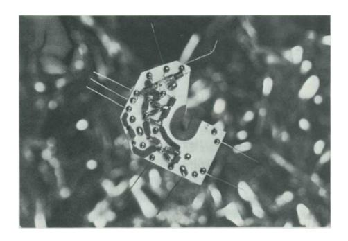
Figure 38: high voltage cascade in ceramic thick-film technology
