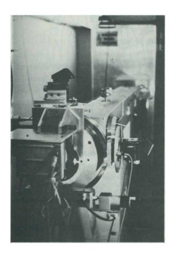
Figure 49: The calibration system for the ion instruments.
