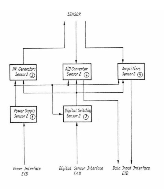
Image 13: Instrument 2 electronics part (block diagram)
