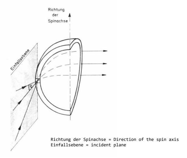
Figure 6: scheme of a quarter sphere electrostatic analyser. Particles with different incidence angles  $\epsilon$  emerge at various points of the Analyzer and then detected with single detectors.
