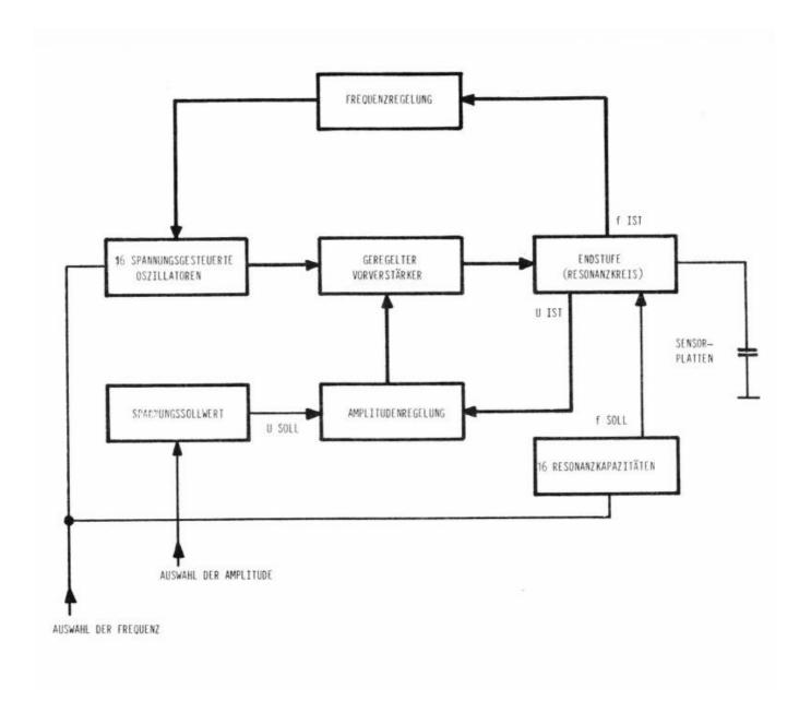
Figure 17: high frequency generator (principle) for instrument I3
