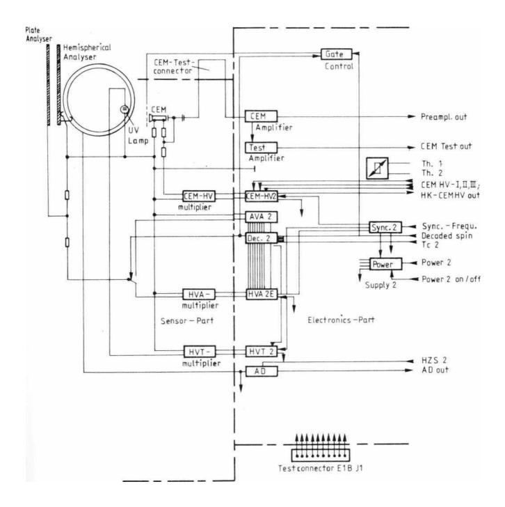
Figure 12: Instrument I2 Block diagram
