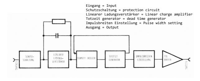
Figure 26: Channeltron amplifier, block diagram
