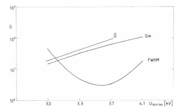
Figure 44: Depending on medium-gain  $\bar{\it G}$ , maximum gain  $G_m$ , as well as the half-width of pulse height distribution of the operating voltage. The recorded measurement on CEM No.163 after permanent load.
