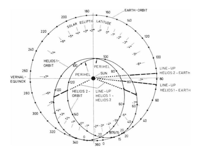
Figure 2: The orbit ellipses from HELIOS 1, HELIOS 2 and the Earth. The day numbers refer to the year 1976.
